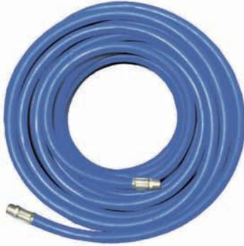
Heavy Duty Hose features a Black Nitrile tube; a Blue Neoprene cover with reinforcement of multiple textile spirals. Designed for air and water, this hose has excellent flexibility. It can be used with reusable fittings or crimped-on barb fittings (pages 22-23). This hose is electrically non-conductive and adheres to a 4:1 Safety Factor and RMA Class A - High Oil Resistance.
