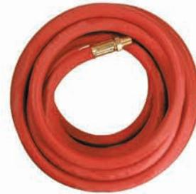
General Purpose Hose features a Black EPDM Tube; Red EPDM Cover with a reinforcement of Multiple Textile Spirals. Designed for air and water applications where contact with petroleum products is minimal. This hose can be used with reusable fittings or crimped-on barb fittings (pages 22-23). It adheres to a 4:1 Safety Factor and RMA Class C - Medium Oil Resistance.
