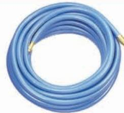
Thermoplastic combines prime PVC with special additives allowing this hose to resist long term deterioration caused by exposure to air line lubricating oils. A tough cover protects against scuffs, cuts and abrasions while rayon spiral synthetic cord assures added strength, making this product a popular choice for industrial environments. Thermoplastic hose should be used with crimped-on barb fittings only (see page 23). Available in Blue and with or without fittings.
