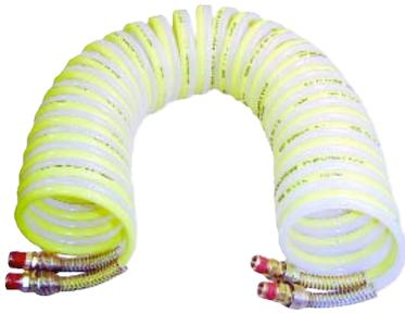
Twin Bonded Self-Storing Nylon Air Hose provides an efficient way to service applications that require air and fluid transport or air and an exhaust return. The intermittent bond allows fittings to be installed without damaging the individual tubes. One yellow tube and one natural colored tube simplify tube identification. Cut-to-length coils are supplied with swivel fittings that have a pre-applied thread sealant. They are also available in 50' bulk coils without fittings.
