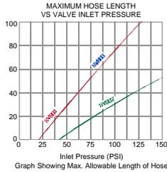
**Note:** Nominal sizes of valve and connecting hose must be consistent (i.e. 1/4" valve to be used with 1/4" hose).
